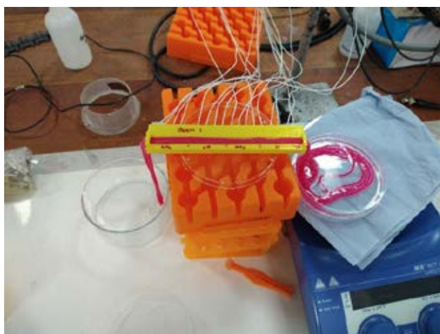
Figure 1: ISEs encased into yellow, 3D-printed case. From left to right, there 4 ISEs for each of ammonium, pH, nitrate, and potassium followed by one reference electrode. Pink threads are wicking fluid from the right hand side using capillary action. The container on the left hand side is used to collect the fluid and evaluate transported nutrients. White wires serve as contact with the data acquisition system.
